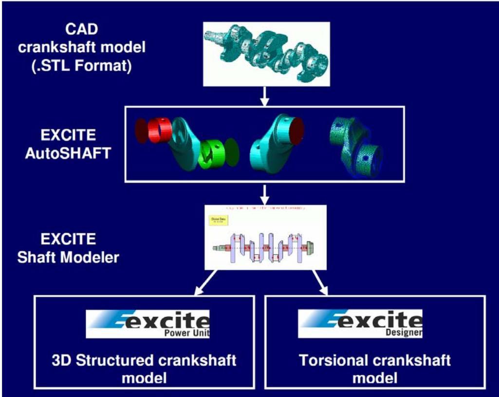
Fig. 8. Flexible crankshaft MBS model for 1D and 3D analysis automated derived from CAD-STL file
